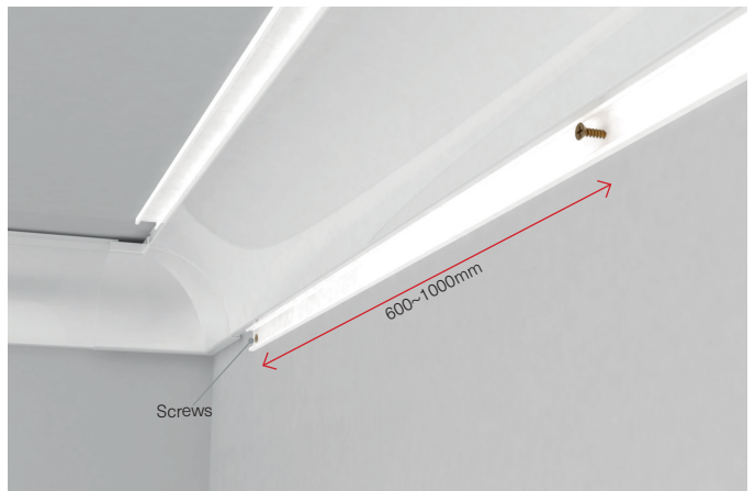
2. The mounting rail should be secured to the wall/ceiling using appropriate fixings every 600~1000mm (2~3')
